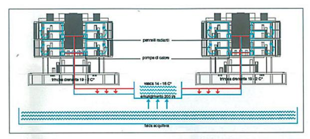
coordination between architectural design and plantengineering allows Tortona 37 to take advantage of the geothermal energy, which is a free source, to create hot and cold water by means of water polyvalent heat pumps, one of the most efficient systems currently available causing the least environmental impact.
